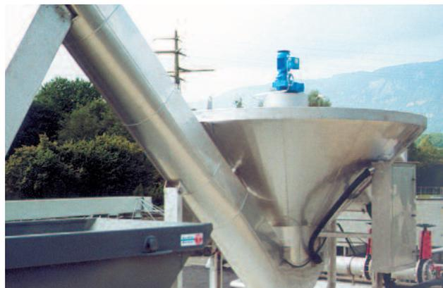
Innovative technology: HUBER Coanda Grit Washer RoSF4 size III, heated plant for outdoor installation
