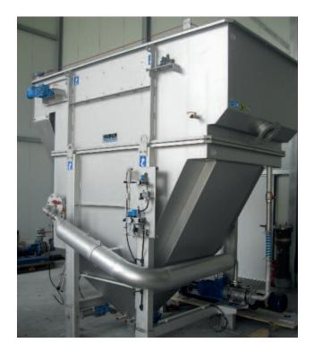
>>> HUBER Dissolved Air Flotation HDF for advanced (waste)water treatment with micro bubbles
