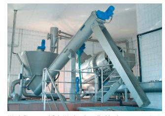
Wash Drum and Grit Washer installed in the customer's building
