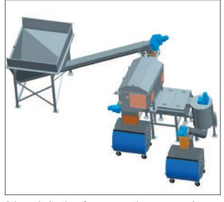
Schematic drawing of a compact grit treatment unit
