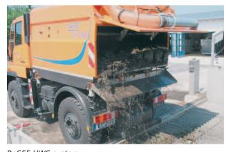
RoSF5 HWS system: Acceptance tank with horizontal dosing screw
