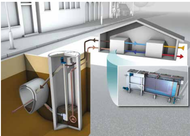
Eco-friendly heat supply for buildings: HUBER ThermWin® with HUBER Heat Exchanger RoWin.
