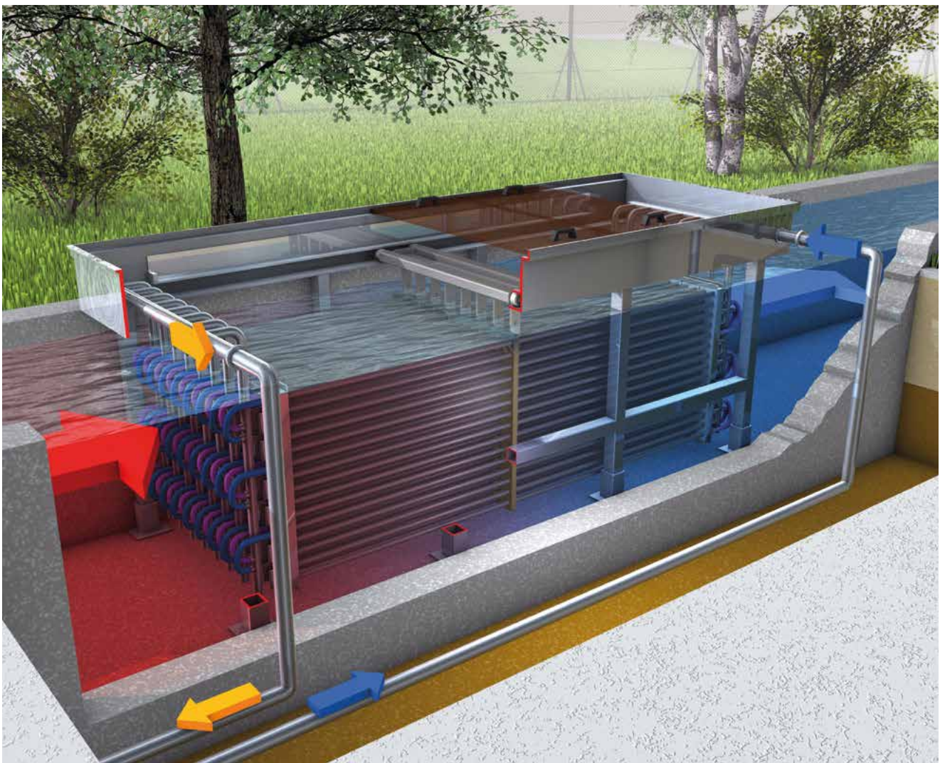
HUBER Heat Exchanger RoWin C installed in a concrete tank. The flow streams through the heat exchanger by gravity.
