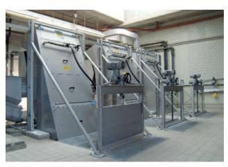
HUBER Fine Screen STEP SCREEN® SSV: 4300 mm long, 3 mm slot width, acid treated in a pickling bath for optimal corrosion protection.
