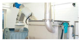
Tank-mounted HUBER Rotary Drum Fine Screen ROTAMAT®...
