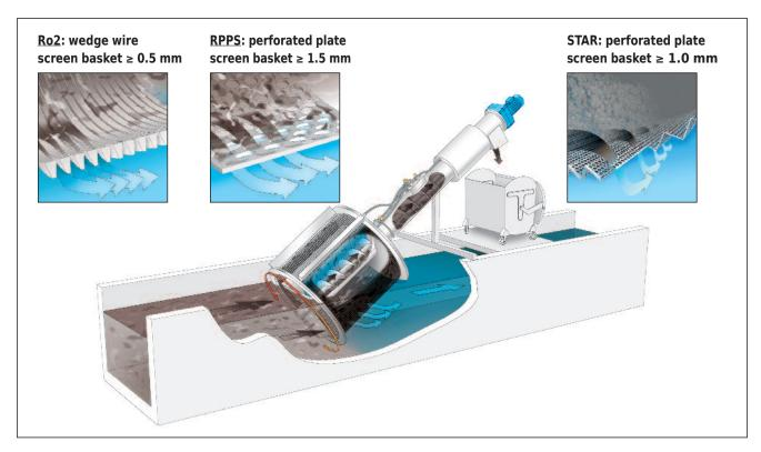
Compared to one-dimensional wedge wire screens (left picture), the two-dimensional screening element of the HUBER Rotary Drum Fine Screen ROTAMAT® RPPS (picture in the middle) achieves a significantly higher separation efficiency.
