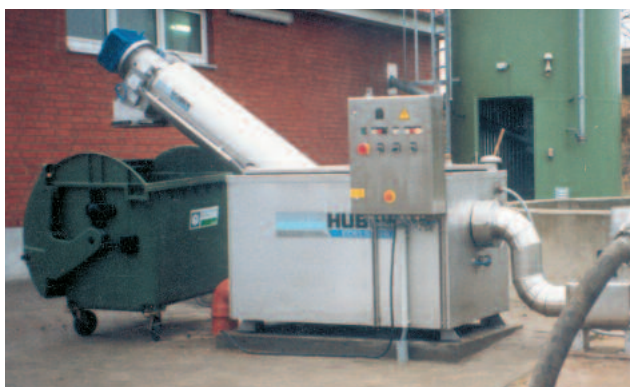
HUBER Sludge Acceptance Plant ROTAMAT® Ro3.1 with HUBER Fine Screen ROTAMAT® Ro1, heated and insulated unit
