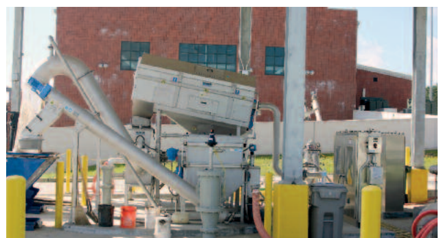
HUBER Sludge Acceptance Plant RoFAS combined with a HUBER Grit Trap ROTAMAT® Ro6
